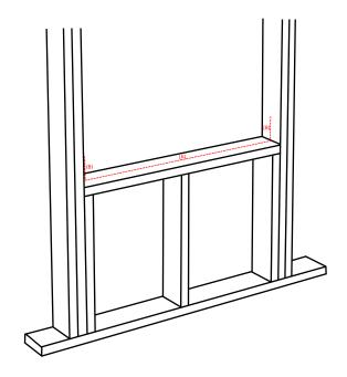
Make relief cuts on each end of Flex-Sill using (B) measurement.
