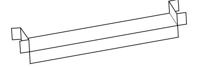
5. Install Flex-Sill pre-formed corners on each side of rough opening.
